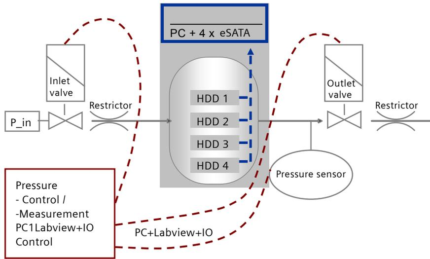
Figure 1: Test setup pressure
