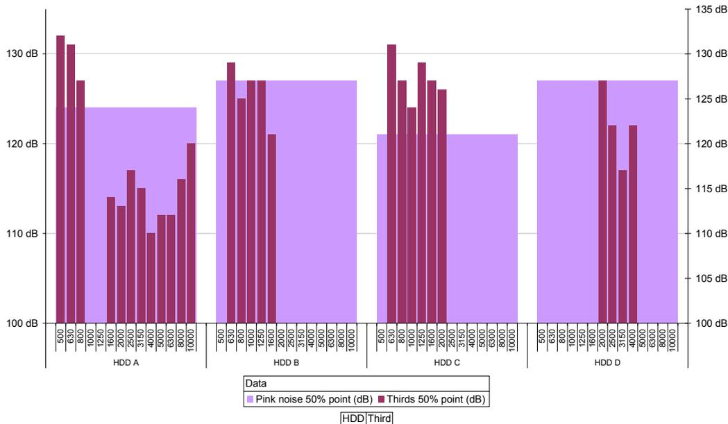
**Figure 3 - Noise Sensitivity of tests HDDs (50% Performance reduction)**
