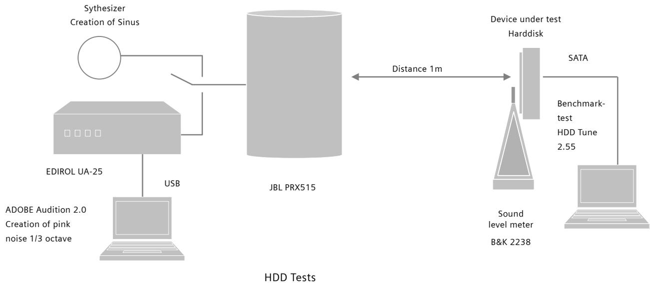
**Figure 2 - Test setup sound**
